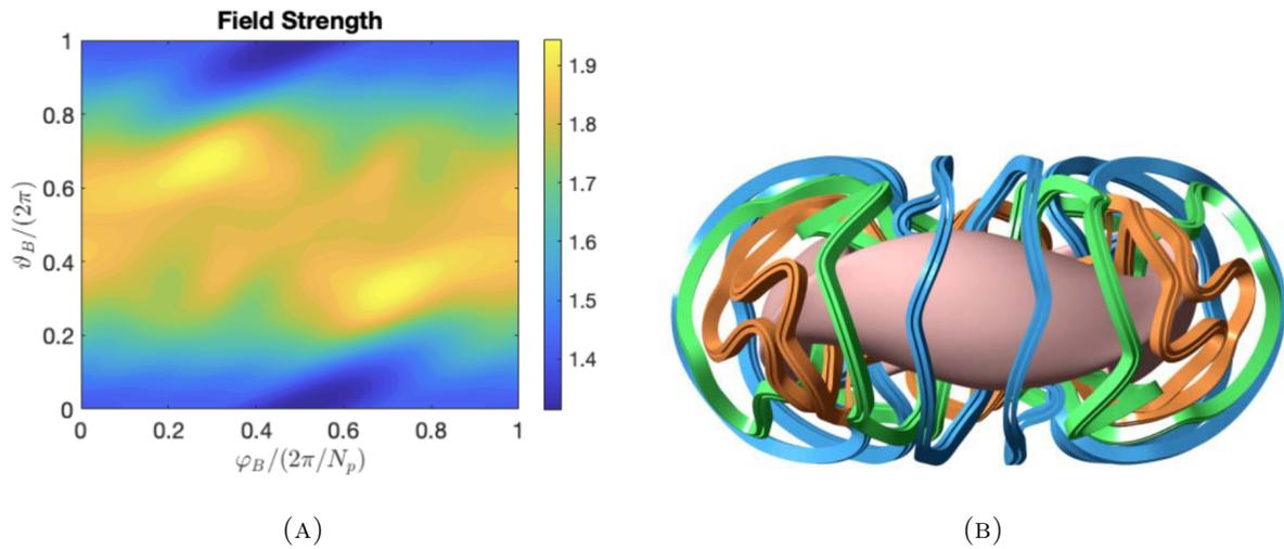
FIGURE 5. The National Compact Stellarator eXperiment (NCSX) (a) field strength and (b) coils with plasma boundary. [D. J. Strickler et al, *IAEA* 2006]
