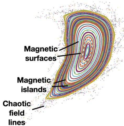
FIGURE 1. Poincaré section of the magnetic field evaluated from the NCSX modular coils. Here a magnetic field is followed many times around a device until it intersects a plane at constant toroidal angle. Colors differentiate different magnetic field lines.
