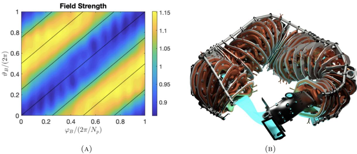
FIGURE 6. The Helically Symmetric eXperiment (HSX) (a) field strength and (b) coils with plasma boundary. [F. S. B. Anderson et al, *Fusion Technology* 1995]
