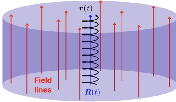
FIGURE 3. The guiding center trajectory (blue) describes the particle's motion (black) after averaging over the fast gyration.
