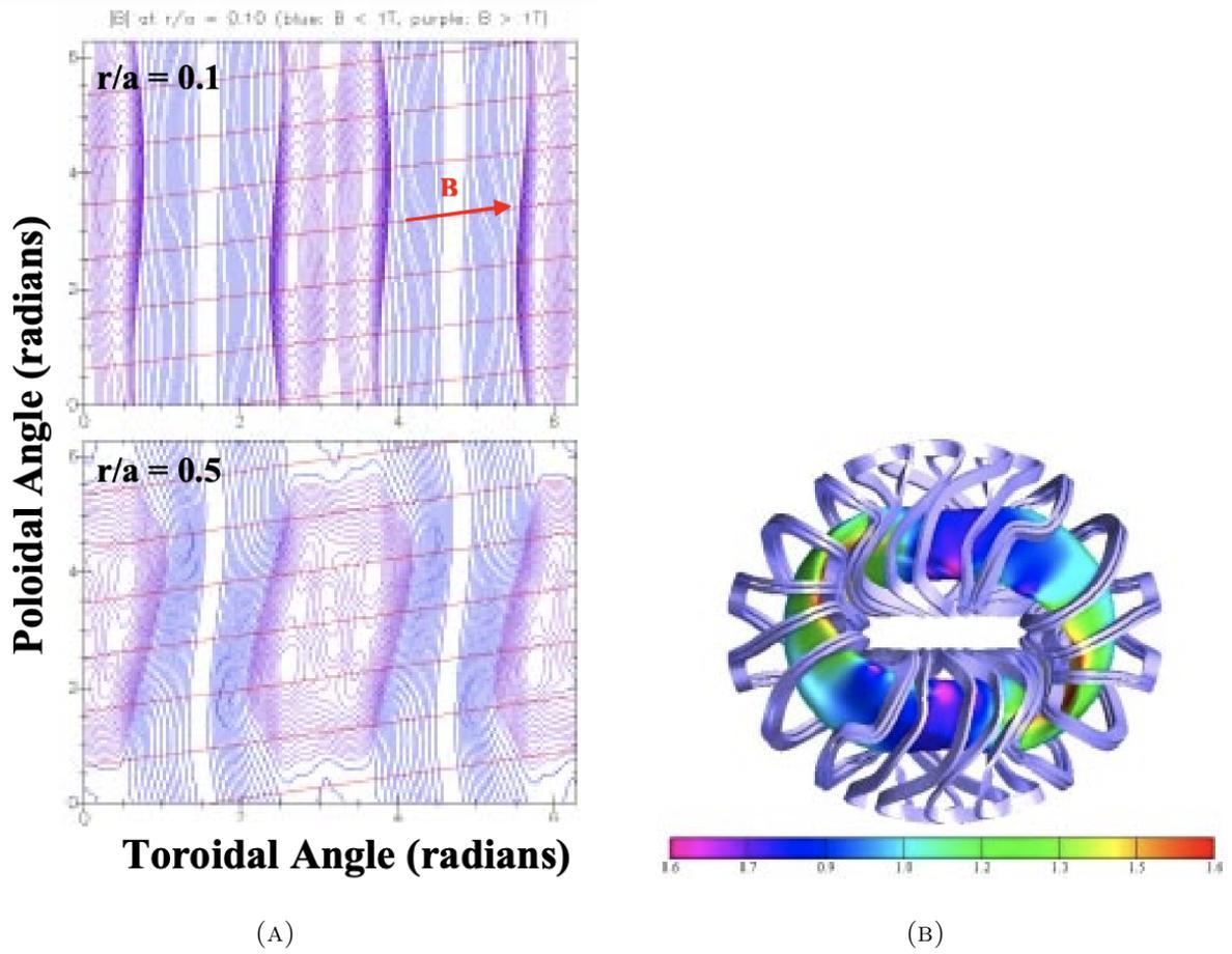
FIGURE 4. The Quasi-Poloidal Stellarator (QPS) (a) field strength and (b) coils with plasma boundary. [J. F. Lyon et al, *IAEA* 2005]
